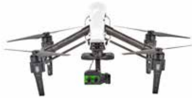
Lock-and-Go Gimbaled Double 4K Sensor on DJI Inspire 1
