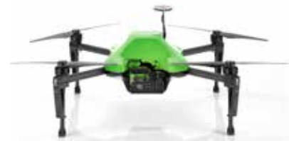
Double 4K Sensor on Sentera Omni
