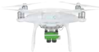
Double 4K Sensor on DJI Phantom 4
