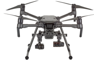
AGX710 and ZENMUSE XT Sensors Mounted on MATRICE 210 Drone
