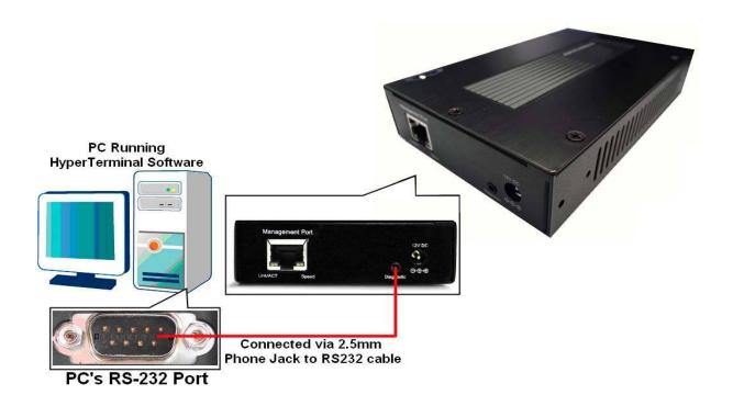
CT-10G-MC series allows users to make system configurations and view test statistics/system information with **HyperTerminal**. To access CT-10G-MC series via **HyperTerminal**, you have to connect CT-10G-MC series' **Diagnostic Port** with **PC's RS-232 Port** via a 2.5mm Phone Jack to RS-232 cable as shown in the figure above.
