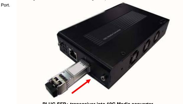
PLUG SFP+ transceiver into 10G Media converter
