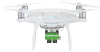
Double 4K Sensor on DJI Phantom 4
