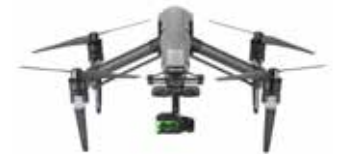
Lock-and-Go Gimbaled Multispectral Double 4K Sensor on DJI Inspire 2 Drone
