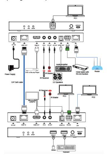
**POC** The CrystalView HDBaseT extender supports PoC power from either end. Simply select the most suitable end to locate the external power supply.
