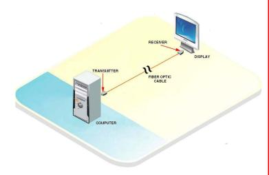
Cables The Transmitter and Receiver are connected using standard single-mode or multi-mode fiber cables, sold separately.
